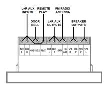
A line level input from an external audio source may be connected to the AUX L & R terminals. These should be fed from the audio source to the WA-215 using shielded 2-core cable. Connect Left+ and Right+ to the AUX L & R terminals and both Left- and Right- to GND.
