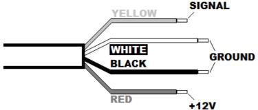
The amplifier can be operated from any 12Vdc power supply capable of delivering up to 1.2A current.
