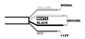
The amplifier can be operated from any 12Vdc power supply capable of delivering up to 2.1A current.
