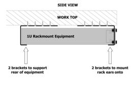
Secure the rack ears through the mounting holes as shown using the supplied screws and hex nuts provided. For 2U models, it is possible to mount a single 2U appliance or 2 x 1U appliances if required.
