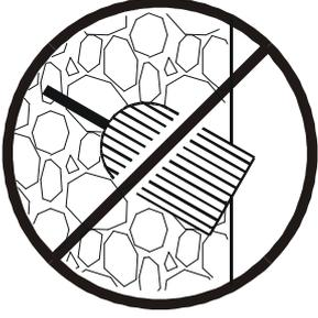
Keep the detector away from dust and dirt, which can cause premature wear of parts.
